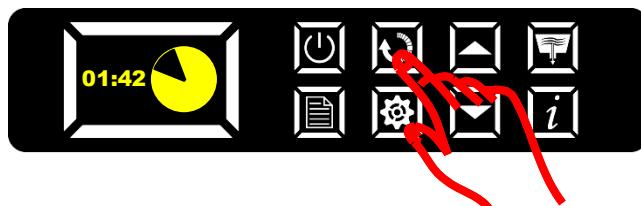
The 10 min cycle can be interrupted at any time by pressing the button (■) again
