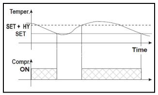
Figure 3-1 - Compressor Temperature Regulation
