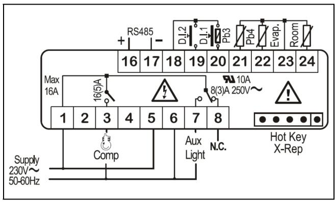
Figure 16-1 - XR35CX Connections
