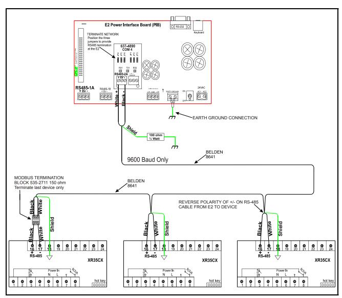
Figure 17-1 - XR35CX to E2 MODBUS Network Wiring
