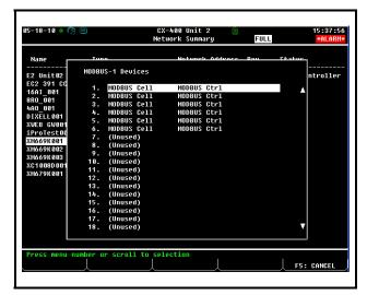
Figure 18-6 - List of MODBUS Devices
