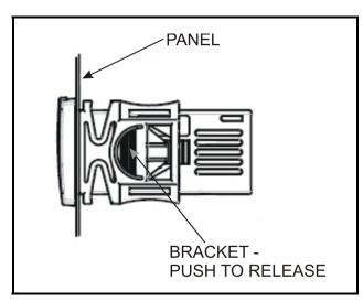
Figure 11-1 - Installation and Mounting of XR35CX
