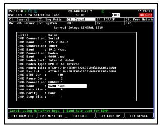
Figure 18-3 - Serial Communications Manager Screen
