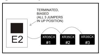
Figure 18-2 - MODBUS Networking
