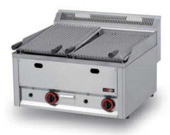
Selection of modules of 330, 660 mm width • Two types of burners with output 4 kW and 6,5 kW • GLS burner is removable, GL is foxed in the burner chamber • The selection of grid for meat or fish • Grid material AISI 304 • 660 mm module contains 2 independent burners • Plate rim (space coverage) is welded on both sides which Guarantees better hygienic conditions • Fat drawer with 1 litre volume • Control only with the regulation knob
