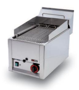
Upper plate thickness 0,8 mm from AISI 304, the rest AISI 430 • Module width 330 mm, 1 heating zone • Heating element material AISI 304 L • GN 1/1 with depth 65 mm • Removable rim around the plate (spillage cover) • Simple control of the electrical variant by means of the main switch and regulation knob • Regulation element is rheostat with positions 0-7 • Simple shifting of electrical box on the guiding bar with safety device to prevent unwanted box extraction
