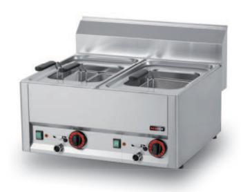
External basin filling. i.e. no water supply • Simple control by means of one regulation knob • The drain is placed in the front part, fitted with a safety clip to prevent unwanted water drainage • Signalling of the heating elements with an indicator • Drain ¾ • The package includes also the fitting extension of the drain for simpler water drainage into the vessel • GN ½ 200 mm • 8 litre volume for one basin • The cookers include the safety thermostat • Safety thermostat: 130 °C
