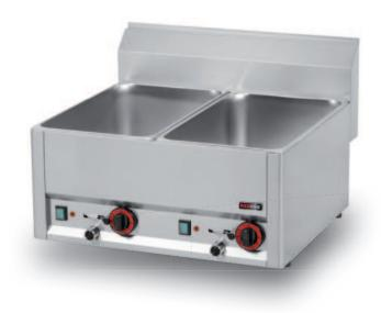
Basin size GN 1/1 with depth 163 mm for inserting GN 150 mm • BM-30 EL one basin, BM-60 EL two basins • Operating thermostat 30-90 °C • External basin filling, i.e. no water supply • Simple control by means of one regulation knob • The drain is placed in the front part, fitted with a safety device to prevent unwanted water drainage • Signalling of the heating elements with an indicator • Drain ¾ • The package includes also the fitting extension for simpler water drainage into the vessel
