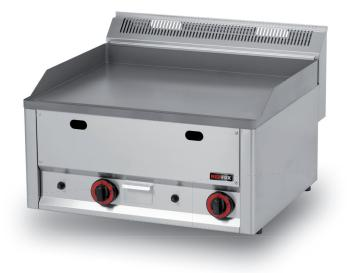
Selection of modules of 330, 660, 990 mm width • The option of several surface variants and the plate materials • Smooth or ribbed surface, the option of surface combination • The plate material is steel or hard chrome steel • Griddle plate thickness is 10 mm – it guarantees smaller temperature fluctuation • Plate rim (space coverage) is welded on both sides • Fat drawer with 1 litre volume • Simple control by means of the main switch and regulation knob
